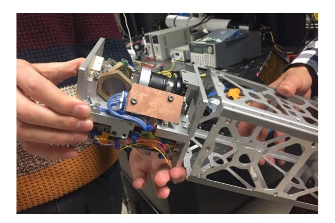
A new laser-pointing platform developed at MIT may help launch miniature satellites called CubeSats into the high-rate data game. Credit: Jennifer Chu
