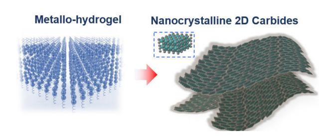
Molecules in gelatin naturally self-assemble in flat sheets, carrying the metal ions with them (left). Heating the mixture to 600 degrees Celsius burns off the gelatin, leaving nanometer-thin sheets of metal carbide. Credit: Xining Zang illustration, copyright Wiley
