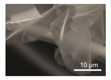
When magnified, the two-dimensional metal carbides resemble sheets of cellphane. Credit: Xining Zang photo, copyright Wiley
