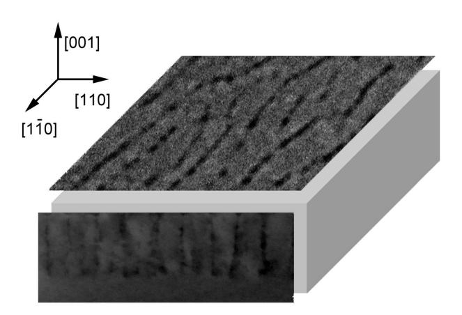
By using lasers, scientists from Germany and Poland were able to create a remarkable compound of indium arsenide and iron. Surprisingly, the compound -- the black stripes in this image -- formed lamellar-shaped structures in the surface of the crystal along one crystalline axis. Credit: HZDR / S. Zhou
