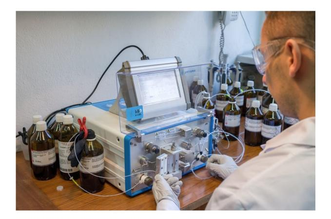
In microfluidic devices, the size of the catalyst nanoparticles can be modified interactively. Credit: IPC PAS, Grzegorz Krzyzewski
