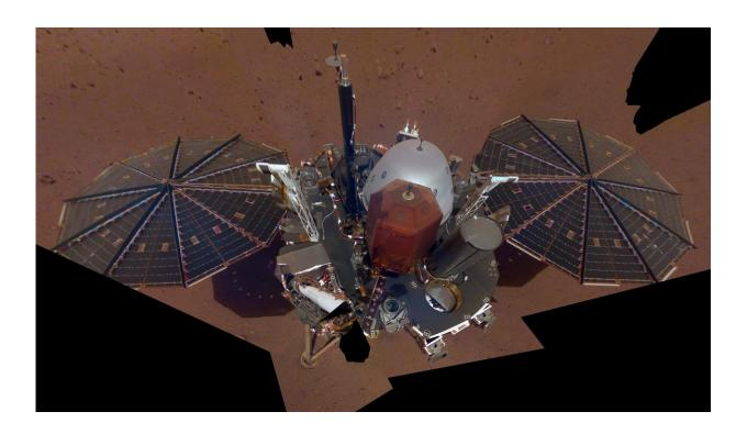
This is NASA InSight's first full selfie on Mars. It displays the lander's solar panels and deck. On top of the deck are its science instruments, weather sensor booms and UHF antenna. The selfie was taken on Dec. 6, 2018 (Sol 10). The selfie is made up of 11 images which were taken by its Instrument Deployment Camera, located on the elbow of its robotic arm. Those images are then stitched together into a mosaic. Credit: NASA/JPL-Caltech
