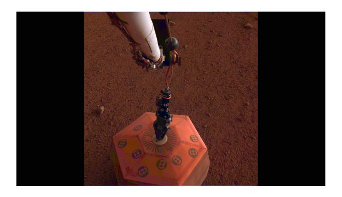
NASA's InSight lander placed its seismometer on Mars on Dec. 19, 2018. This was the first time a seismometer had ever been placed onto the surface of another planet. Credit: NASA/JPL-Caltech
