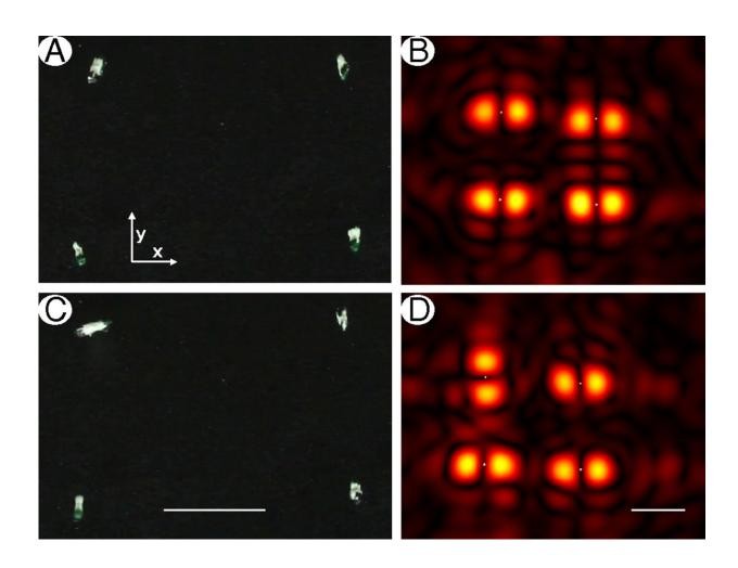
Individual orientation of asymmetric particles trapped above a reflective surface with an array placed 15.1  $\lambda$  (13 cm) above it. (A) All EPS particles aligned along the y axis; (C) one EPS particle is orientated along the x axis. (B and D) Corresponding simulated pressure amplitude at the reflecting surface. (Scale bar, C and D: 2 cm.) Credit: *Proceedings of the National Academy of Sciences* (2018). DOI: 10.1073/pnas.1813047115
