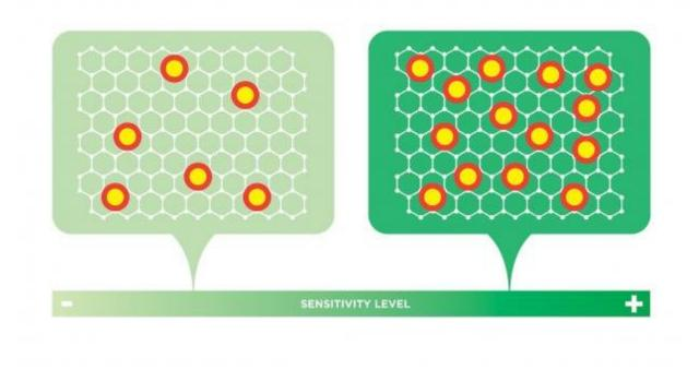
NYU researchers discovered how to predict the sensitivity of graphene electrodes — potentially paving the way to industrial-scale production of the ultra-small sensors: The density of intentionally introduced point defects is directly proportional to the sensitivity of the graphene electrode. If the density of these points is maximized, an electrode can be created that's up to 20 times more sensitive than conventional electrodes. Credit: NYU Tandon School of Engineering
