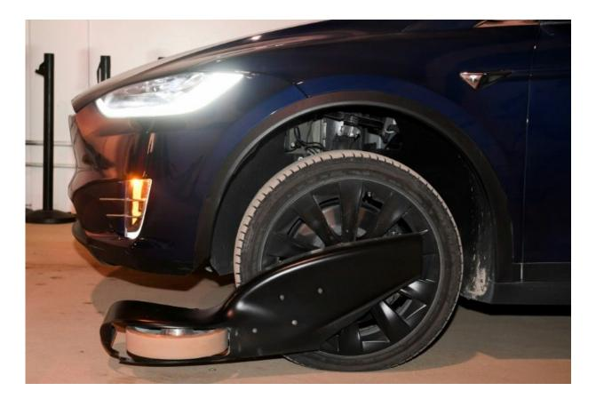
Cars are fitted with tracking wheels which stabilize the vehicle on a track allowing them to travel at high speed through a tunnel
