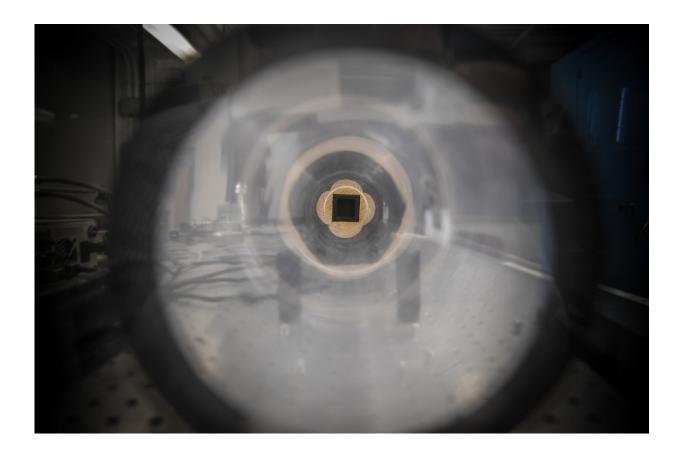
In Thomas's lab at NJIT, mosquitoes are placed in a tube enclosure where they transit through a laser beam and reflect distinct signatures of backscattered light. Credit: NJIT
