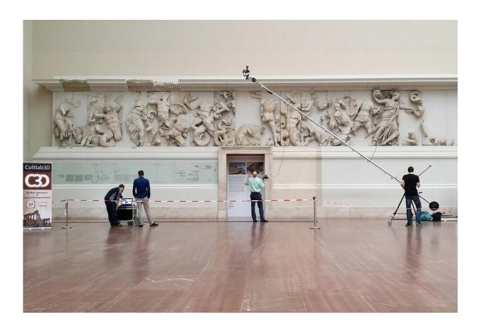
Researchers use a laser scanner to scan the frieze of the Pergamon Altar. Credit: Fraunhofer IGD
