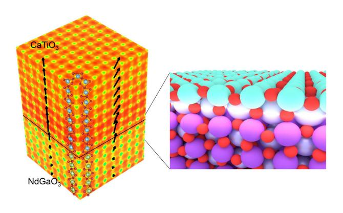
A reconstruction of a perovskite crystal (CaTiO3) grown on a similar perovskite substrate (NdGaO3) showing electron density and oxygen octahedral tilt. (insert) Artist's conception of the interface between substrate and film. Credit: Yakun Yuan/Penn State
