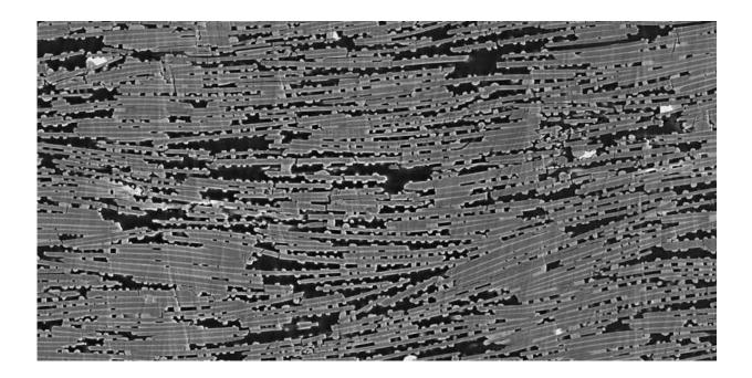
A cross-section of a mother-of-pearl imitation shows that at temperatures of 800 degrees Celsius and above, nubs form between the platelets, which solidify the material. Credit: Kunal Masania / ETH Zurich
