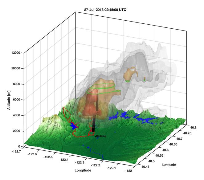
"3D rendering of radar reflectivity isosurfaces at 29 (red), 24 (orange), 20-10 (gray shades) dbZe. The vortex center locations are shown as the solid black line. The cloud base heights are shown as green contours." Credit: University of Nevada, Reno
