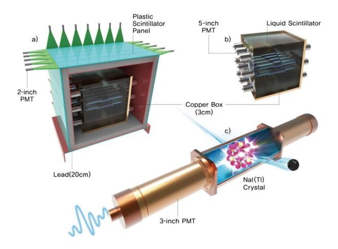
The detector is contained within a nested arrangement of shielding components shown in schematic a). The main purpose of the shield is to provide full coverage against external radiation from various background sources. The shielding components include plastic scintillator panels (blue), a lead brick enclosure
