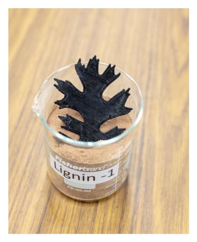
Using as much as 50 percent lignin by weight, a new composite material created at ORNL is well suited for use in 3D printing. Credit: Oak Ridge National
