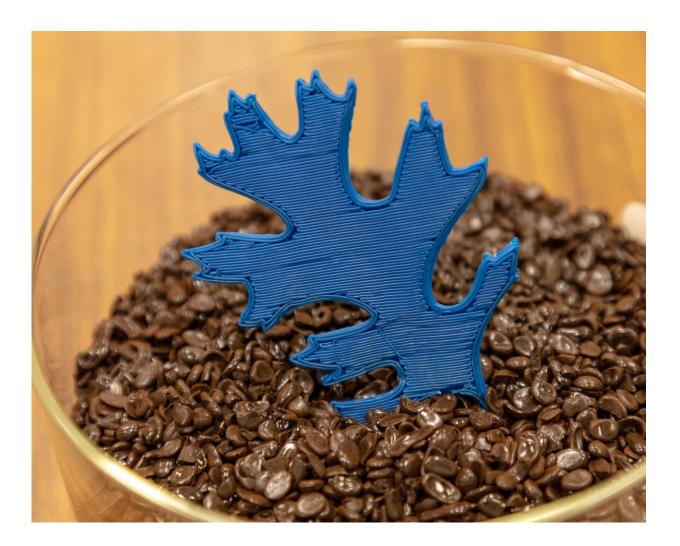
A new composite of lignin and nylon is easily extruded during 3D printing and exhibits good mechanical strength in finished products. Credit: Oak Ridge National Laboratory
