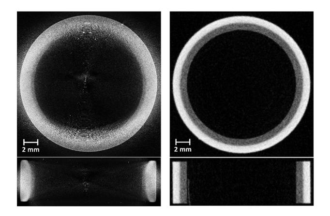
Example of cross sectional tomography data slices from the xy (top) and xz (bottom) planes for the ITER\_MB\_ROI sample with a comparison of X-ray (left) vs. neutron (right) tomography imaging results. Credit: Llion Evans, Swansea University
