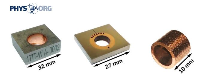
Three sample types used for this work: (left) ITER reference monoblock (ITER\_MB), (centre) Culham Centre for Fusion Energy thermal break concept monoblock (CCFE\_MB) and (right). Credit: Llion Evans, Swansea University
