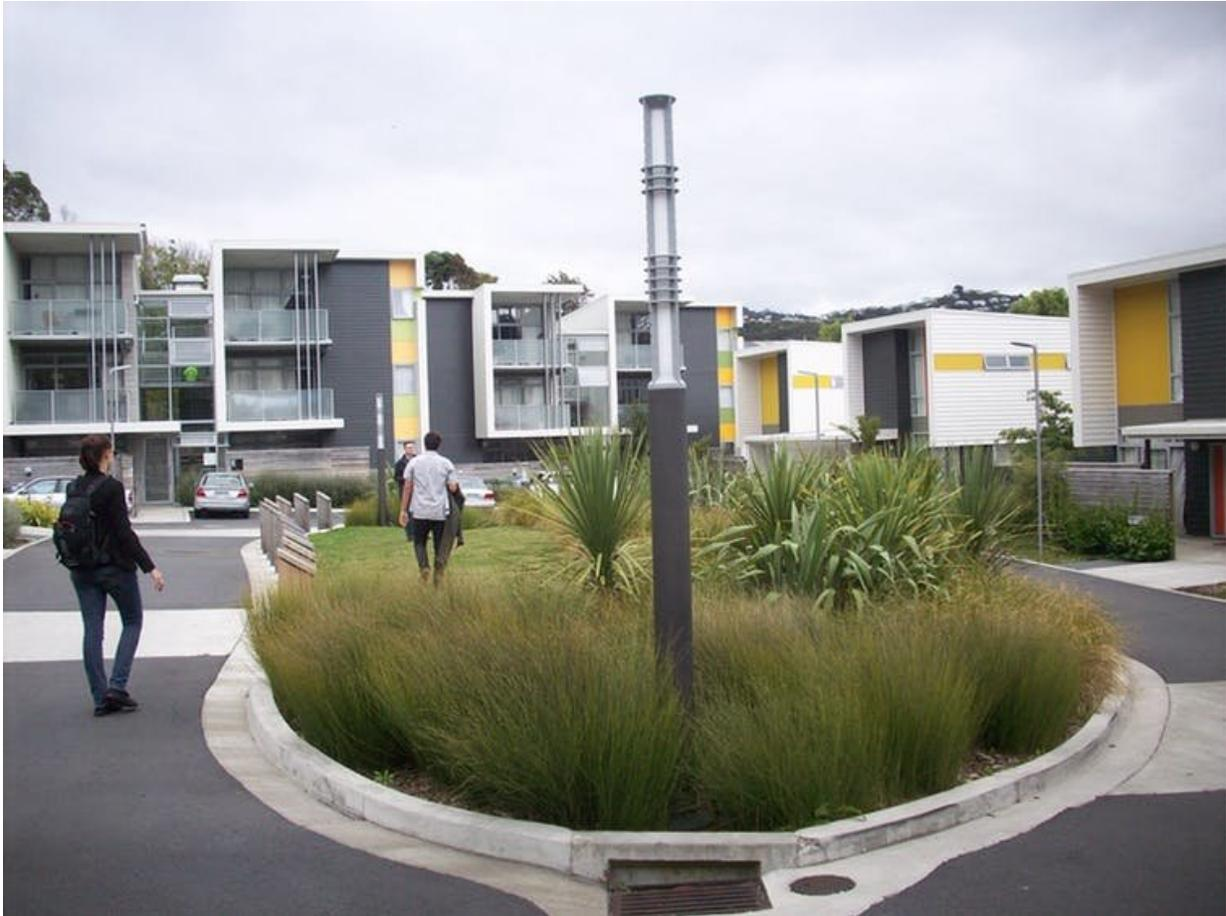
A rain garden, which absorbs rain and stores water to help control run-off from impervious hard surfaces, in Wellington, New Zealand. Credit: Karine Dupré
