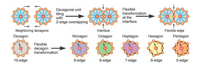
Researchers from Brown University have shown that a particular type of nanoparticle building blocks can assemble themselves into a quasicrystalline superlattice. The researchers showed that the particles form decagons (10-sided polygons), which them stitch together to form a lattice. The researchers showed that in order to fill in space in the lattice, the decagons flex into with polygons with five-nine sides. Credit: Chen Lab / Brown University
