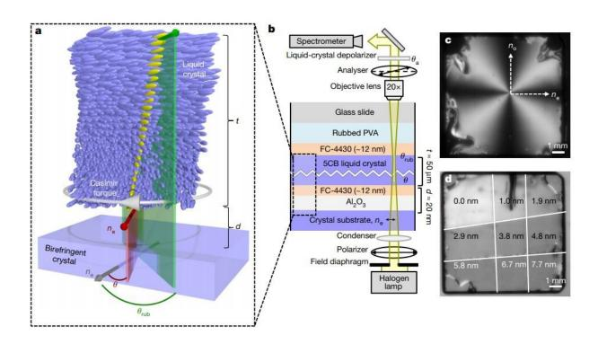
Apparatus measuring the Casimir torque. Credit: *Nature* (2018). DOI: 10.1038/s41586-018-0777-8
