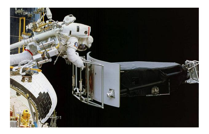
Astronaut Jeffrey Hoffman removes the Wide Field and Planetary Camera 1 (WFPC 1) during the first Hubble servicing mission (SM1), which took place in December 1993. Credit: NASA
