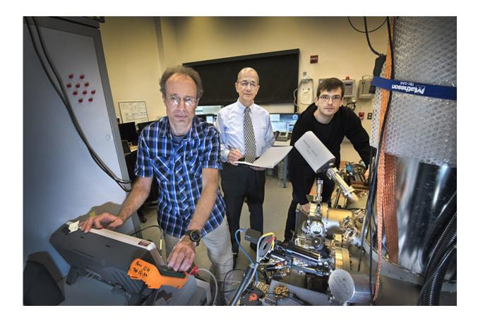
Brookhaven Lab scientists Percy Zahl (left), Ivan Bozovic (center), and Ilya Drozdov at the Center for Functional Nanomaterials. Here, they used a custombuilt scanning tunneling microscope to image the surface structure of twodimensional atom-thin sheets of boron on copper. Credit: Brookhaven National Laboratory
