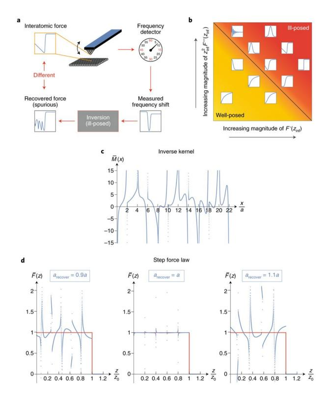
Frequency-modulation force spectroscopy. a, Flow chart of an ill-posed measurement. b, Master plot of practical force laws of different shape (white boxes) and their position in the ill-posedness phase space. c, Inverse kernel,
