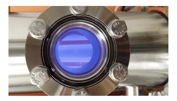
CO2-rich planetary atmosphere exposed to a plasma discharge in Sarah Hörst's lab. Credit: Chao He
