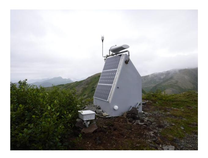
Transportable Array station P19K is one of the closest stations to the Iniskin earthquake origin. Solar panels power the station, and the seismometer is buried in a specially drilled borehole to insulate it from surface noise. Photo taken in 2017 during a service site visit by Incorporated Research Institutions for Seismology (IRIS). IRIS manages the Transportable Array station installation and maintenance. Credit: Doug Bloomquist, IRIS
