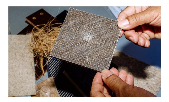
A section of date palm fiber composite used in the mechanical testing. Credit: University of Portsmouth
