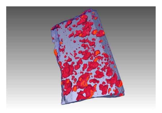
An X-ray tomography image (CT scan) of an ore sample showing frozen droplets of sulfide liquid as red blobs. Credit: Steve Barnes, Author provided
