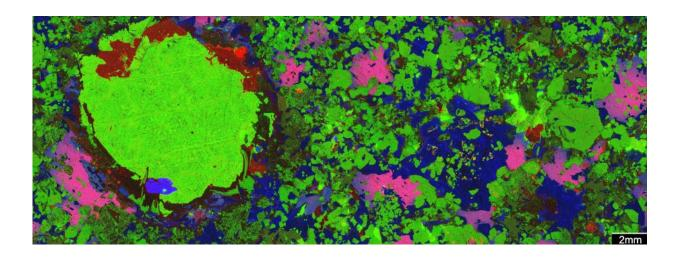
The green blob is metal-rich molten sulfide in an ore from the Norilsk area in Siberia, the most valuable accumulation of metals of any kind on the planet. Credit: Steve Barnes, Author provided
