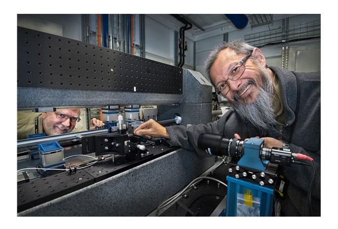
NSLS-II scientists Scott Coburn (left) and Wah-Keat Lee (right) are shown at the Full Field X-ray Imaging beamline, where scientists and engineers have built a transmission x-ray microscope that can image samples 10 times faster than previously possible. Credit: Brookhaven National Laboratory
