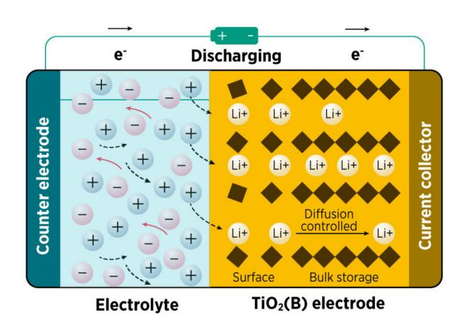
A titanium dioxide electrode takes in lithium ions as the battery discharges. Credit: Ref. 1. © 2018 Wiley-VCH Verlag GmbH & Co. KGaA, Weinheim
