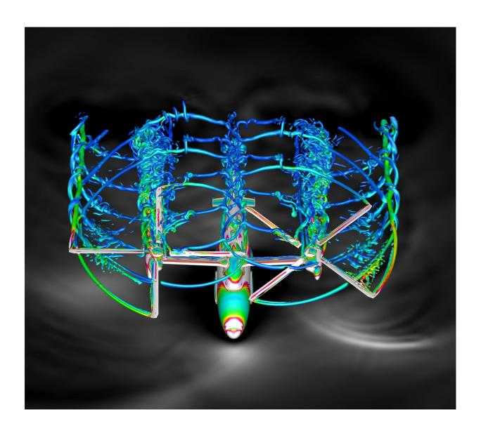
Visualization of NASA's side-by-side rotorcraft concept for UAM in forward flight. This back view shows the complex 3D vortex wake from the intermeshing
