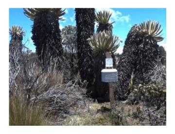
The team has installed 23 sensors to track temperature, relative humidity, and dew point every hour at altitudes of up to 16,000 feet. Credit: Sarah Fecht
