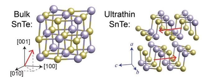
Schematics of the spontaneous polarization of bulk SnTe (left) and ultrathin SnTe (right). Credit: University of Arkansas
