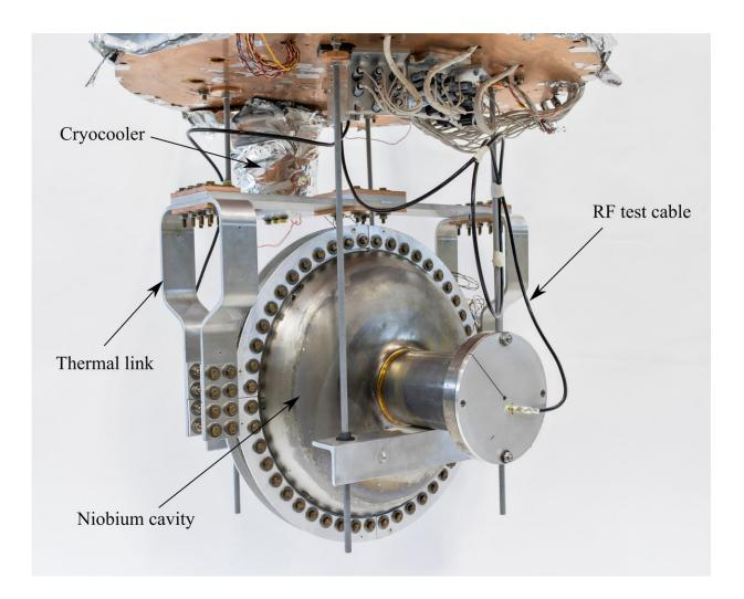
A superconducting radio-frequency accelerator cavity is mounted and connected to a cryocooler, cooling the cavity without the use of liquid helium. This new device could make it easier to produce high-average-power electron beams for industrial applications. Credit: Marty Murphy
