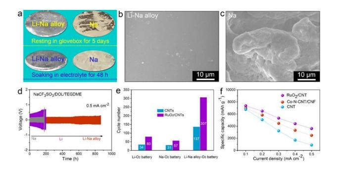
a) Comparison of oxidation and corrosion resistance of Li-Na eutectic alloy and Na metal. SEM images for Li-Na alloy b), and Na c) electrodes after five stripping/plating cycles. d) Voltage profiles for symmetric metal batteries. Cycling e), and rate f) performance of metal-O2 batteries with and without catalysts Credit: YAN Junmin, ZHANG Yu, ZHANG Xinbo
