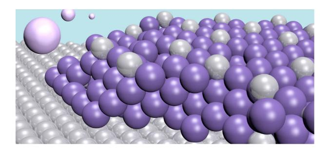
When mercury ions (light purple) in a liquid come near an electrode of platinum, they are attracted to the electrode's surface where they get reduced to metallic mercury. On the electrode, mercury atoms (dark purple) and platinum atoms (grey) develop into a very strong alloy, and the mercury is thus removed from the water. Credit: Björn Wickman and Adam Arvidsson/Chalmers University of Technology
