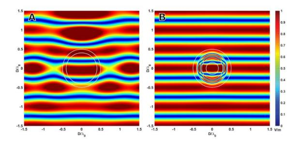
Interaction of light with a hollow sphere of silicon (A) and with the same sphere filled with a potion composed of three different strata (B). Credit: UEx
