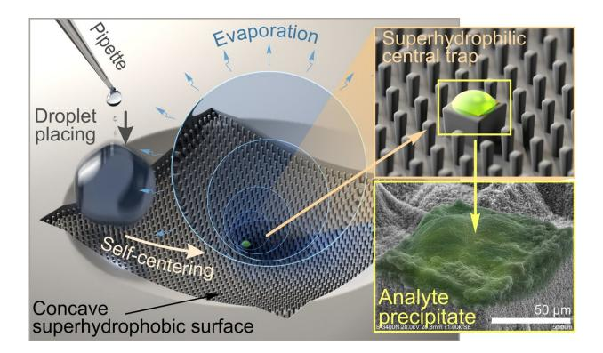
Picture explaining how the concentrator platform works. Credit: 'Nanotechnologies' scientific educational center, FEFU
