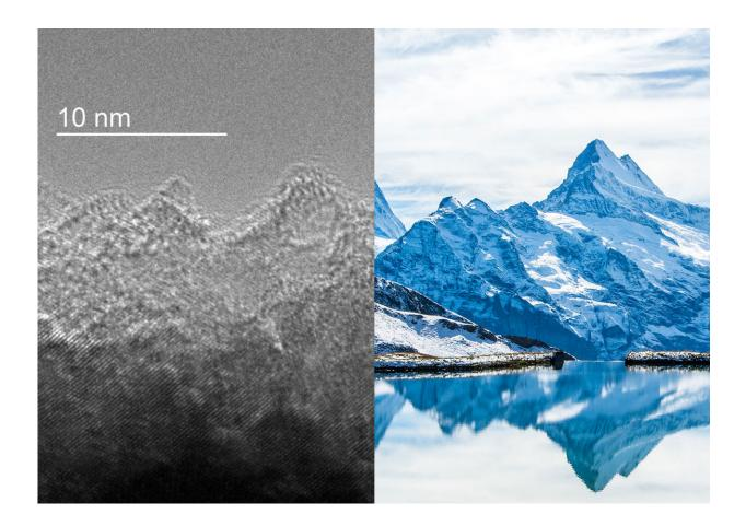
The surface of the nanodiamond material (left) was measured at the atomic-scale using a transmission electron microscope. The local slope was found to be steeper than that of the Austrian Alps (right) measured at the scale of a human. Credit: Tevis Jacobs
