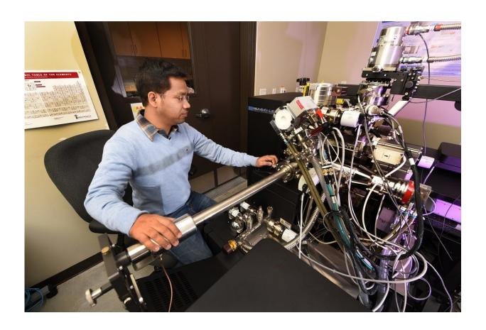
INL materials scientist Subhashish Meher uses a local electron atom probe at the Center for Advanced Energy Studies to study the microstructure of treated superalloys. Credit: Idaho National Laboratory
