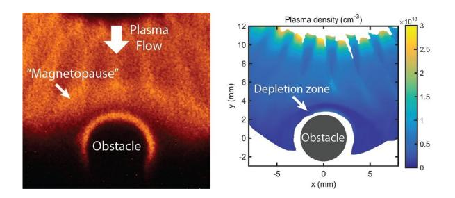
Optical images from MAGPIE experiments (left) show a detached boundary, reminiscent of Earth's magnetopause, formed when a model solar wind encounters a magnetized obstacle. A plasma depletion zone is seen surrounding the body (right) due to the shielding effect of the field. Credit: MAGPIE group, Imperial College London
