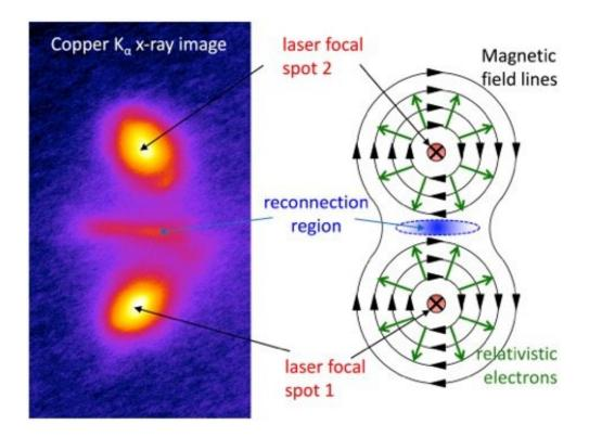
(top) Experimental x-ray image showing the laser heated spots and a third bright region in the center where magnetic reconnection takes place. (bottom) An illustration of the magnetic field geometry. Credit: Center for Ultrafast Optical Science, University of Michigan
