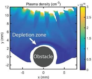
Optical images from MAGPIE experiments (left) show a detached boundary, reminiscent of Earth's magnetopause, formed when a model solar wind encounters a magnetized obstacle. A plasma depletion zone is seen surrounding the body (right) due to the shielding effect of the field. Credit: MAGPIE group, Imperial College London
