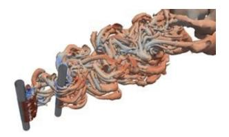
Modelling vortices in an ocean current around two cylinders could help marineoffshore engineers design better risers. Credit: A\*STAR Institute of High Performance Computing
