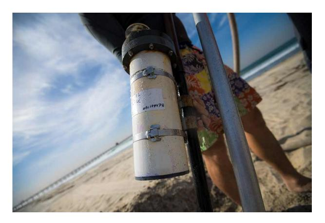
Three pressure sensors will be installed at the mean high-water line throughout Imperial Beach. The sensors will be retrieved after winter to collect and analyze the data. Credit: Erik Jepsen/UC San Diego Publications
