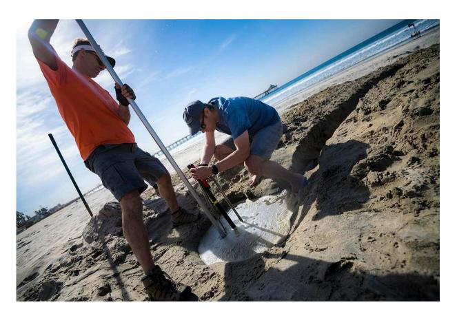
Researchers with the Center for Climate Change Impacts and Adaptation at Scripps install pressure sensors in the sand in Imperial Beach on Nov. 13, 2018. These sensors will assess the wave run-up predictions in flood-prone areas. Credit: Erik Jepsen/UC San Diego Publications
