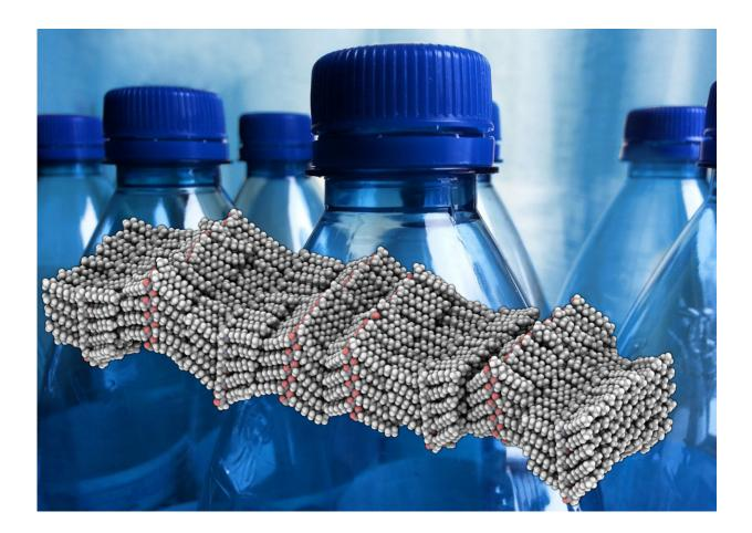
A rendering (gray and pink) of the molecular structure of a peptoid polymer that was studied by a team led by Berkeley Lab and UC Berkeley. The team's success in imaging the atomic-scale structure of polymers could inform new designs for plastics, like those that form the water bottles shown in the background. Credit: Berkeley Lab, Charles Rondeau/PublicDomainPictures.net
