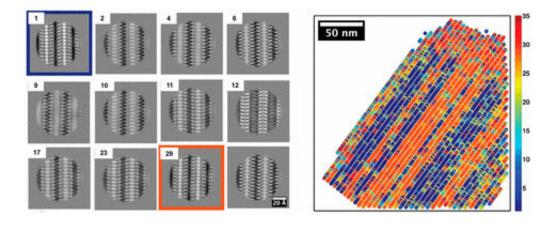
Researchers developed a colorized map (right) to show the distribution of different types of crystal structures (left) that they found in the polymer peptoid sample. The scale bar in the map image is 50 nanometers, or 50 billionths of a meter. Credit: Berkeley Lab, UC Berkeley
