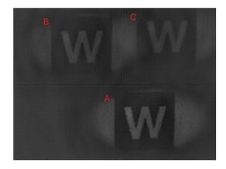
A block letter W imaged by three different prototype metalenses (A, B and C) using different mathematical models — both without (left) and with (right) computational postprocessing. Credit: <u>Liu et al.</u>, <u>Nano Letters</u>, <u>2018</u>
