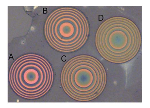
Four ultrathin metalenses developed by University of Washington researchers and visualized under a microscope. Credit: <u>Liu et al., Nano Letters, 2018</u>
