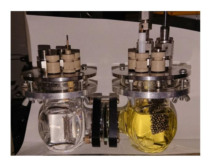
The CO2 reduction reaction takes place in the cathodic chamber shown on the right. Credit: *Chemical Science*
