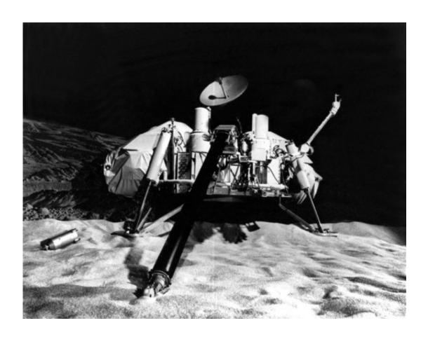
This undated photo shows NASA's Viking lander in a Mars simulation laboratory. The two cylinders on the top of the Lander are survey cameras, and below the right hand camera is one of 3 rocket motors used during the final soft landing on Mars. Viking 1 was launched on Aug. 20, 1975 and arrived at Mars on June 19, 1976. Viking 2 was launched Sept. 9, 1975 and entered Mars orbit on Aug. 7, 1976. The twin Vikings were the first successful landers on Mars from planet Earth. (AP Photo)
