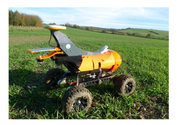
A farming robot named "Tom" produced by Small Robot Company as part of a field trial to develop new farm technologies, in East Meon, southern England, Friday Nov. 30, 2018. The "agri-tech" startup company is developing lightweight autonomous machines that can carry out precision "seeding, feeding and weeding" in the hope of transforming food production. (AP Photo / Kelvin Chan)
