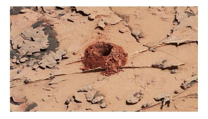
This NASA image shows a 2-inch-deep hole the rover Curiosity drilled on the Martian surface to extract rock samples in May 2018
