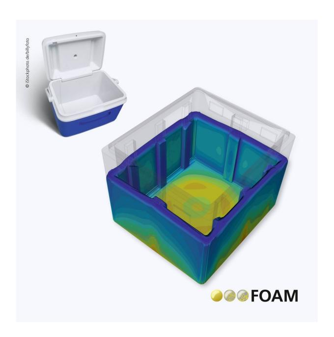
PU expansion simulation with FOAM for manufacturing a cooler. Credit:
