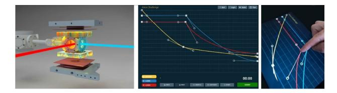
Game interface of the Alice Challenge. Players could manipulate three curves representing two laser beam intensities and the strength of a magnetic field gradient, respectively. The chosen curves were then realized in the laboratory in real-time. Credit: Robert Heck, AU
